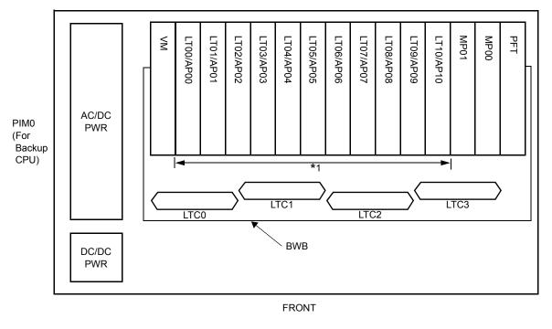
LT00-LT10 : Line/Trunk card mounting slots AP00-AP10 : Application Processor card mounting slots MP00/MP01 : PN-CP27-A mounting slot VM : PZ-VM00/VM00-M/VM03-M mounting slot PFT : PZ-8PFTB mounting slot AC/DC PWR: PZ-PW121/PW126 mounting slot DC/DC PWR: PZ-PW122 mounting slot
